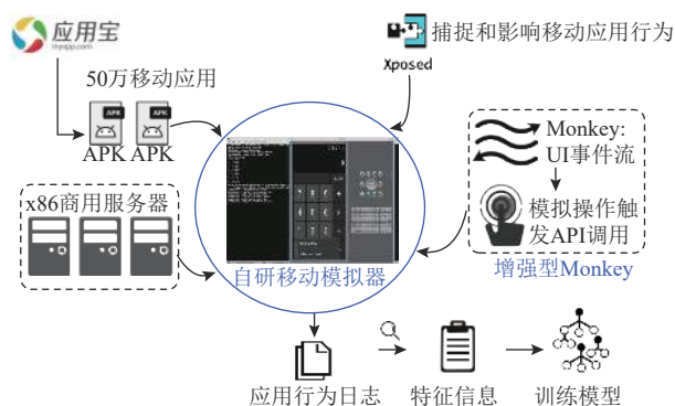
Fig. 14 General workflow of intelligent security detection system for Android Apps
