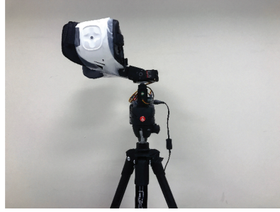
Fig. 9. Our VR testbed consists of a GearVR, an S7, a Pan/Tilt mount, a 3D-printed holder for the mount, a Raspberry Pi to accurately control the mount's motion, and a tripod for stabilizing the test instruments.
