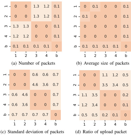
Fig. 12. Fisher’s discriminant ratio matrix for four features. Each element in the matrix represents the Fisher’s discriminant ratio of the Orvibo Light’s interactions corresponding to the horizontal and vertical coordinates. Large values mean significant difference between the two interactions.
